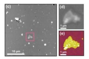
"Laser targeting" for nanoscale microscopy: On the left, a typical 900 square micrometer view, using focused laser beam, shows potentially interesting purple membrane patch, which is marked with the square. Right top, closer optical image of patch; bottom, same target imaged with AFM revealing topological detail. Credit: A.B. Churnside, University of Colorado at Boulder
