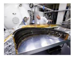
Northrop Grumman lead venting analyst Dan McGregor inspects a sunshield test article for the sunshield section on top of the spacecraft around the tower that
