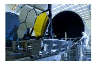
The chamber is opened to move the first cryogenically tested gold-coated engineering development unit out of Marshall's X-ray and Cryogenic Facility. Each of the 18 mirror Webb telescope primary mirror segments will be tested, repolished, coated with gold, measured at Ball Aerospace, and finally tested again in the Marshall test facility at cryogenic temperatures before the mirror test program is complete. (NASA/MSFC/Emmett Given)
