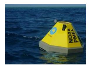
A mooring with a suite of ocean acidification and other environmental sensors at Heron Island on the Great Barrier Reef is the latest tool in an expanding global network of ocean measurements, informing scientists of changes in ocean chemistry. Credit: Dr. Bronte Tilbrook, CSIRO, Australia
