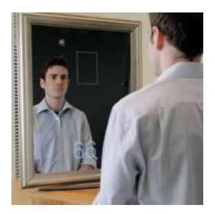
MIT Media Lab student Daniel McDuff, who collaborated on the pulsemonitoring system, demonstrates a version of the device built into a mirror that displays his pulse rate in real-time at the bottom. Image: Melanie Gonic
