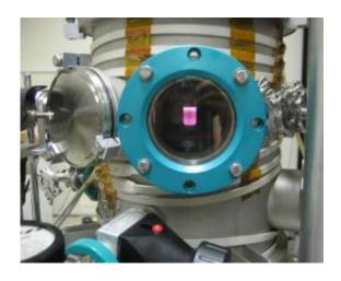
A window into Titan's atmosphere: Energized by microwaves, the gas mix inside the reaction chamber lights up like a pink neon sign. Thousands of complex organic molecules accumulated on the bottom of the chamber during this experiment. (Photo: S. Hörst)
