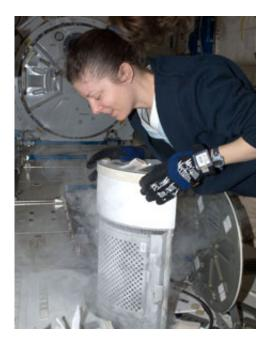
NASA astronaut Tracy Caldwell Dyson, Expedition 24 flight engineer, replaces a dewar tray containing biological samples in the Minus Eighty Degree Laboratory Freezer for ISS in the Kibo laboratory of the International Space Station. Image Credit: NASA
