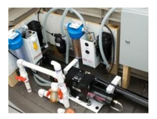
In the system, a solar photovoltaic panel powers pumps that push seawater through a permeable membrane to remove salt and other minerals. Photo: Melanie Gonick
