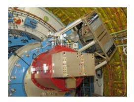
Cornell University's Faint Object Infrared Camera for the SOFIA Telescope, or FORCAST, is shown attached to the SOFIA telescope. (NASA / Tony Landis)
