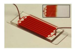
The herringbone pattern of interior surfaces in the HB-Chip brings more circulating tumor cells into contact with the antibody-coated capture surfaces. The inset shows the uniform blood flow through the device. Credit: *Proceedings of the National Academy of Sciences*
