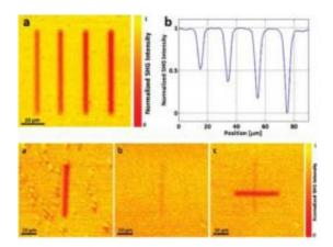
(Top) The image in (a) shows lines written using the photodimerization technique, corresponding to lower SHG signals in (b). (Bottom) These images show a line that was (a) written, (b) erased, and (c) rewritten perpendicular to the first line. Image credit: Iliopoulos, et al. © 2010 American Chemical Society.
