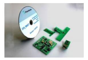
By means of the evaluation kit consisting of a motherboard, two antennas for UHF and MW range and software, users can develop their own solutions. (© Fraunhofer IPMS)
