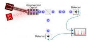
In new NIST experiments, the "color" (wavelength) of photons from a quantum dot single photon source (QD SPS) is changed to a more convenient shade using an up-conversion crystal and pump laser. To test that the process truly acts on single photons without degrading the signal (by creating additional photons), the output is split in two and sent to parallel detectors -- true single photons should not be detected simultaneously in both paths. Credit: NIST
