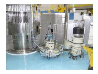
The Cold Triple Axis spectrometer, now in commissioning at Oak Ridge National Laboratory's High Flux Isotope Reactor, moves by way of air pads on an epoxy surface known as the "dance floor."
