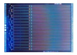
Integrated circuit for NIST's new programmable AC/DC 10-volt standard. The chip contains about 300,000 superconducting Josephson junctions (located along horizontal lines at right-center of micrograph). Credit: NIST
