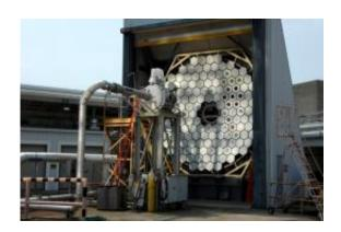
The Solar Thermal Test Facility's concentrator mirror is composed of 144 smaller hexagonal segments. When all the mirrors are fully uncovered, the mirror beams about 1,000,000 watts per square meter of solar energy intensity into the vacuum chamber at the focal point. (NASA/D. Oliver)
