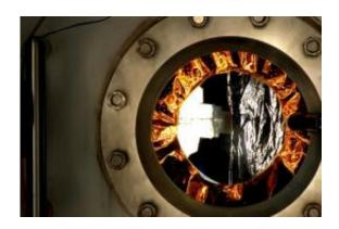
Engineers put the instrument inside this vacuum chamber where the pressure is lowered to the vacuum conditions of space. The black liquid nitrogen cooled walls simulate the super-cold conditions space has to offer. The sun is illuminating the front of the instrument bright white. (NASA/D. Oliver)
