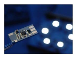
Siemens is developing magnetic ceramic films so that the highperformance electronic circuits used in lighting systems and other such devices can be made smaller and much easier to manufacture. This type of circuit adapts the voltage, current, and frequency to the electrical consumer, for instance, a lamp.
