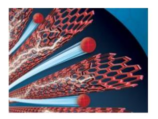
By aligning carbon nanotubes inside polymer composites, Wardle and his colleagues designed electrodes that allow ions to travel more quickly between the tiny cylinders. Image: Joe Klimek, Lazerpro Digital Media Group
