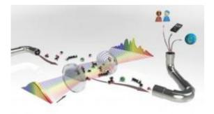
This is an artist's rendering of JILA's molecular fingerprinting system. A gas mixture (left) is probed by a frequency comb, a laser-based tool for identifying different colors of light. By analyzing the amounts of specific colors absorbed, the system quickly identifies molecules and their concentrations. Applications may include diagnosing disease, detecting security threats, and measuring trace gases in the atmosphere. Credit: Baxley/JILA
