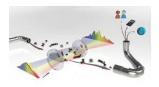
This is an artist's rendering of JILA's molecular fingerprinting system. A gas mixture (left) is probed by a frequency comb, a laser-based tool for identifying different colors of light. By analyzing the amounts of specific colors absorbed, the system quickly identifies molecules and their concentrations. Applications may include diagnosing disease, detecting security threats, and measuring trace gases in the atmosphere. Credit: Baxley/JILA
