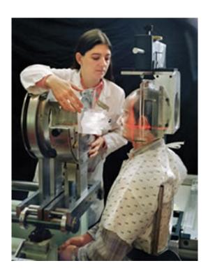
Cancer patients were treated at the Bevalac with the help of a plastic head positioner and beam compensator.
