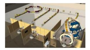
Of three treatment rooms in the Heidelberg Ion-Beam Therapy Center, the one on the right uses a massive gantry that can steer and direct the beams to the patient from almost any angle.
