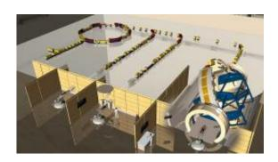
Of three treatment rooms in the Heidelberg Ion-Beam Therapy Center, the one on the right uses a massive gantry that can steer and direct the beams to the patient from almost any angle.
