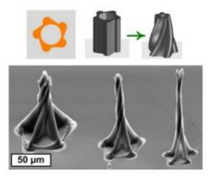
Twisting spires are one of the 3-D shapes researchers at the University of Michigan were able to develop using a new manufacturing process. Credit: A. John Hart
