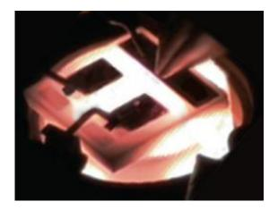
Researchers studied the electrochemical properties of a model fuel cell operating at extreme heat, using a new system for ambient-pressure x-ray photoelectron spectroscopy at the Advanced Light Source.
