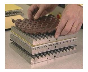
Pressure testing a sealing system: the drainage material (white) and sealing surface (yellow) are clamped between a smooth and a studded pressure plate.
