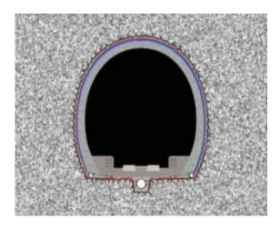
Sealing a tunnel to prevent the ingress of groundwater at high pressure is no easy task. In the NRLA tunnel the drainage system of a shotcrete outer shell, drainage material (red), sealing surface (blue) and load-bearing concrete inner shell must have a service life of about 100 years.
