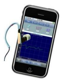
Swiss company CSEM has created the Pulsear device to monitor ones heart rate while exercising. Pulsear uses a tiny unit embedded in a regular earphone to see how fast the pulse is by sending the infrared signals through the tissues in your ear. The result is shown on an iPhone. Pulsear is based on space technology developed to examine how astronauts will behave during long space voyages. Credits: CSEM
