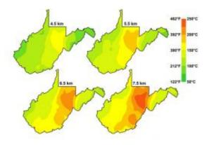
This illustration demonstrates subsurface temperatures at various depths in West Virginia from 4.5 km to 7.5 km, indicating the hottest geothermal resources for further exploration.
