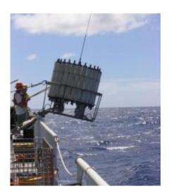
To obtain microbe samples, scientists on the R/V Kilo Moana oceanographic research ship lower a rosette holding 24 bottles that capture samples at different ocean depths in the Pacific Ocean. Photo: Maureen Coleman
