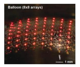
Optical image of an 8x8µ-ILEDs array on a thin PDMS substrate in its on state under deformed conditions. Image credit: *Nature Materials*, doi:10.1038/nmat2879
