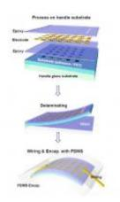
Schematic illustration of the encapsulation of an implantable array of  $\mu$ -ILEDs. Image credit: *Nature Materials*, doi:10.1038/nmat2879
