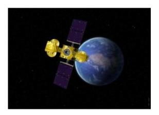
The Hylas-1 telecommunications satellite will operate from from geostationary orbit above the Atlantic at 33.5° West. This first 'Highly Adaptable Satellite' contains an advanced communications payload allowing it to provide broadband internet access to consumers and businesses across Europe as well as supporting a range of conventional telecommunications applications and services. Credits: ESA/S. Corjava
