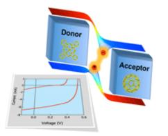
Current-voltage characteristics and energetics of coulombically-bound charge carrier pairs (copper phthalocyanine and boron subphthalocyanine chloride donors, and a fullerene acceptor) at the heterojunction in nanoscale organic semiconductor junctions.
