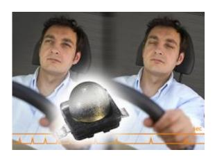
A new infrared light-emitting diode (IR-LED) from the Siemens subsidiary Osram Opto Semiconductors is designed to help recognize the hazardous microsleep that affects motorists. In addition to the IR-LED, this requires a suitable camera with a CMOS sensor. The sensor detects IR light at a wavelength of 850 nanometers, which isn't visible to the human eye, and analyzes the image of the driver that is captured by the camera. And it all takes place unnoticed by the driver - even at night.
