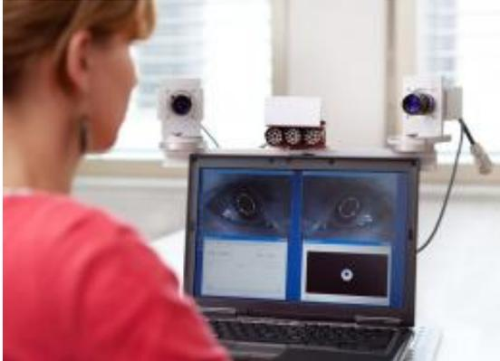
The Integrated Eyetracker developed by the Fraunhofer IDMT permits contact-free and completely calibration-free 3-D measurement of a person's line of vision. (© Fraunhofer IDMT)
