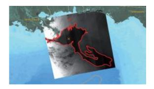
This Envisat Advanced Synthetic Aperture Radar (ASAR) image, acquired on 18 May 2010, shows the extent of the oil spill (outlined in red) in the Gulf of Mexico, following the explosion of the Deepwater Horizon oil rig off the coasts of Louisiana and Mississippi, USA, on 22 April. Credits: GeoVille, ESA
