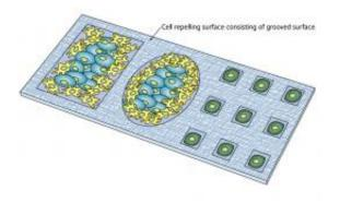
Figure 1: Cells can be corralled on a chip in different ways by etching grooves into its surface. Depending on the area and shape of non-etched areas, cells can be separated and cultured either singly or in clumps of different forms. Credit: 2010 Hiromi Miyoshi
