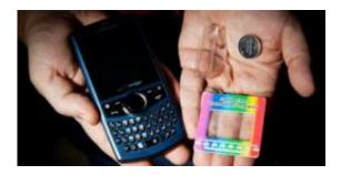
A few basic, inexpensive components and a cellular pone are all high school students need to build a spectrometer, a widely used analytical chemistry instrument. Credit: L. Brian Stauffer, University of Illinois
