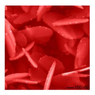
These silver nanoplates are decorated with silver oxy salt nanoparticles along the edges. These nanostructures were grown under irradiation of high-energy x-rays, which allowed scientists to "watch" them grow in real time. The image is from a scanning electron microscope.
