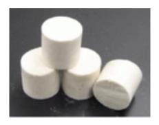
Lighter-than-a-feather, this new material, made from milk protein and clay, could become a new bio-degradable substitute for traditional foamed plastics. Credit: Tassawuth Pojanavaraphan
