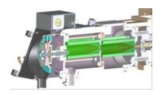
Agilent's new iFunnel ESI-MS interface consists of a multicapillary (6X600 um) inlet and dual ion funnels. An offset between the multicapillary inlet and the first high pressure ion funnel is used to reduce chemical background.
