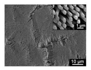
A scanning electron microscope image from an etched section through one of the new alloys. The magnified image inset shows rods of copper 300 nm in diameter emerging from a copper-lanthanum matrix. Image provided by Mark Aindow
