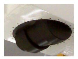
The mounting frame and rotating drum that holds the AirMSPI camera are visible in this view of the underside of the ER-2's forward payload bay. (NASA JPL photo)
