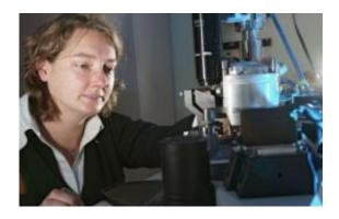
Dr. Stephanie Hoeppener is working with a atomic force microscope for which a Jena researcher team has developed a new procedure allowing to produce sharper probes. Credit: Jan-Peter Kasper/University Jena
