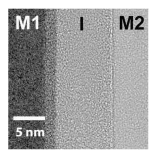
This image of an asymmetric MIM diode reflects a major advance in materials science that could lead to less costly and higher speed electronic products. (Image courtesy of Oregon State University)
