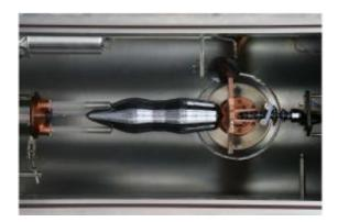
The float-zone 28Si crystal. To determine its density, two spheres were manufactured from the two bulges. To determine the lattice parameter, an X-ray interferometer was cut from the material between these spheres. Image credit: arxiv.org/abs/1010.2317
