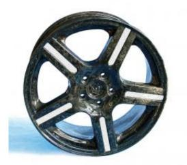
This wheel made of fiber-reinforced plastic is particularly light and exhibits high structural durability. (© Fraunhofer LBF)
