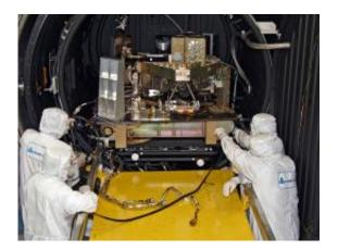
An engineering test unit of the Fine Guidance Sensor is about to undergo cryogenic testing at the David Florida Lab in Canada. Credit: CSA, COMDEV
