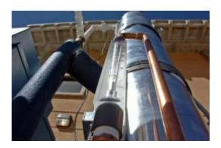
The innovative patent-pending, fluidized-bed sludge drying tower processes 20 pounds of wastewater sludge an hour in a continuous feed system that when developed in full scale is expected to supply the entire electrical needs of the local medium-size wastewater plant. Credit: Photo by Mike Wolterbeek, University of Nevada, Reno
