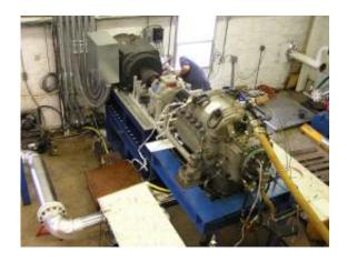
SwRI has designed a test loop for evaluating compressor performance under wet gas conditions.
