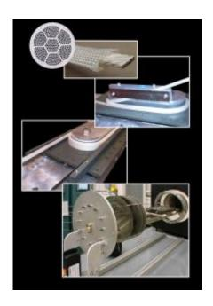
In the process called "wind and react," Bi-2212 wire - shown in cross section, upper right, with the powdered superconductor in a matrix of silver - is woven into flat cables, the cables are wrapped into coils, and the coils are gradually heated in a special oven (bottom).
