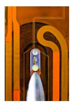
A close-up view of a superconducting magnet coil designed at Berkeley Lab, which may used in a new kind of high-field dipole magnet for a future energy upgrade of CERN's Large Hadron Collider. (Photo Roy Kaltschmidt)
