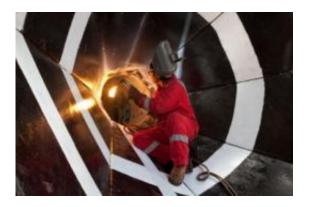
A welder works on a "reentry cone" used to guide drill pipe into the ocean floor. Credit: IODP
