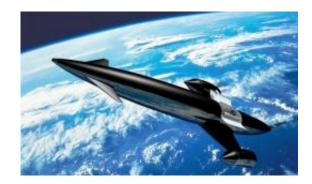
Skylon can reach speeds of up to Mach 25 and altitudes of up to 460 km (285 miles). Image credit: Reaction Engines.
