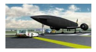
Skylon takes off and lands on a normal runway, reducing the launch cost. Image credit: Reaction Engines.
