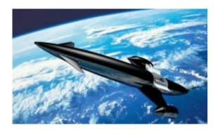
Skylon can reach speeds of up to Mach 25 and altitudes of up to 460 km (285 miles). Image credit: Reaction Engines.
