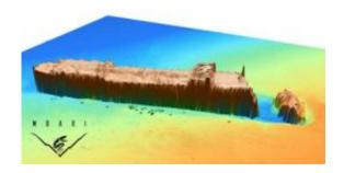
This image, created using sonar data from MBARI's seafloor mapping AUV, shows the wreck of the S. S. Montebello, about 275 meters (900 feet) below the sea surface. The bow of tanker is to right. An amazing amount of detail can be seen, including remnants of the ship's forward mast.
