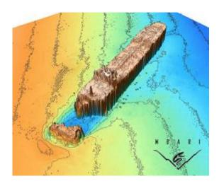
This sonar image shows the bow of the S. S. Montebello, which broke off when the ship sank to the seafloor. The image also includes bottom contours that indicate the shape of the surrounding seafloor.
